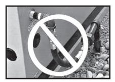
Never bend the flexible fuel line to avoid using an elbow. Bending the flexible line decreases its ability to absorb vibrations and defeats its purpose.
